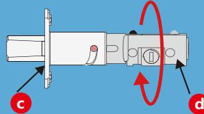
II. Hold the metal plate (c) and twist the deadbolt body (d) clockwise till it snaps to 2-3/8"
