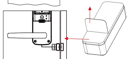
**NOTE:** The arrows must be aligned or as closed as possible (less than 3/4"). If needed, adjust the position of the sensor magnet using provided foam pads to ensure the Lockly logo blinks red when door opens or closes.
