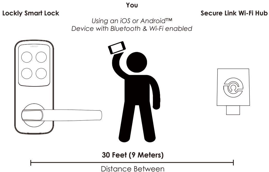
**TIP:** The Secure Link requires a strong wireless signal for optimal performance. Make sure the Secure Link will be installed in a location with a strong 2.4 Ghz wireless signal. Sometimes distances between Wi-Fi hub and lock can vary due to circumstances. If you are having difficulty setting up optimal range of 30/ft or less, we're here to help. Call our customer care team: (669) 500 8835, or visit [Lockly.com/help](https://www.lockly.com/help) for suggestions and troubleshooting tips.
