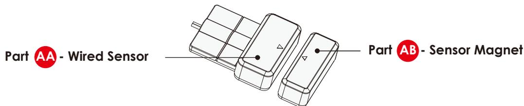
**IMPORTANT: Gap must be less than 3/4" when installed.**
