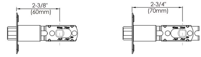
Measure distance between the center of the hole to the edge of door, adjust latch F to 2-3/8" (60mm) or 2-3/4" (70mm)
