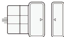
When installed on door, the distance between the wired sensor and sensor magnet must be less than 3/4" in order for the sensor to work. If door frame is higher than door, add included foam pads to level parts **AA** and **AB** with each other as much as possible.
