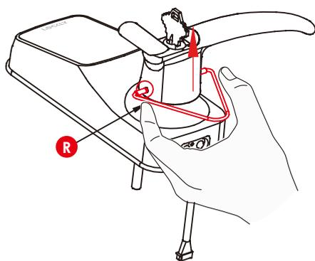
With both dots aligned, use the provided clamping tool **R** to push in the two metal pins at the base of the lock handle located at the 3 o'clock and 9 o'clock positions. Once depressed, remove the handle.
