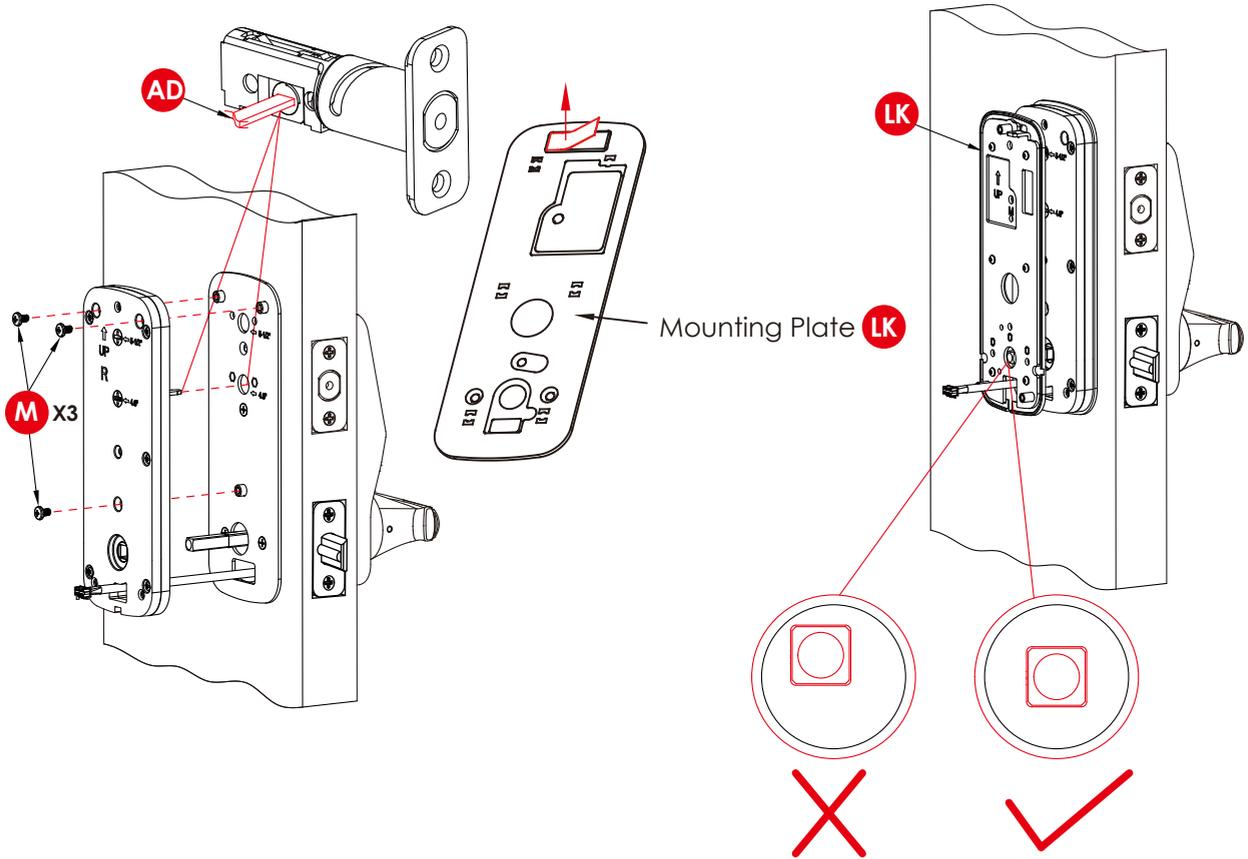
**4** Install plate **P** onto door. Ensure the torque blade **AD** is inserted horizontally to the deadbolt. The spindle must pass through the plate. Secure the plate with screws **M**.
