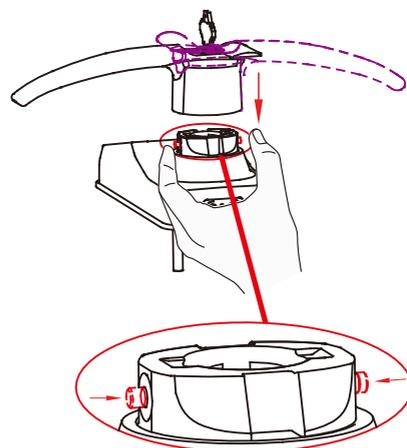
Rotate the handle 180° to the other side of the lock.
