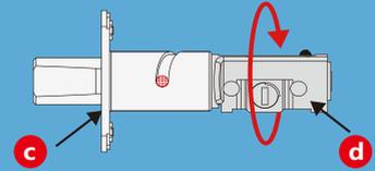
III. To return to default status, while the deadbolt (b) is extended, hold the metal plate (c) and twist the dead bolt body (d) counter-clockwise till it snaps to 2-3/4"
