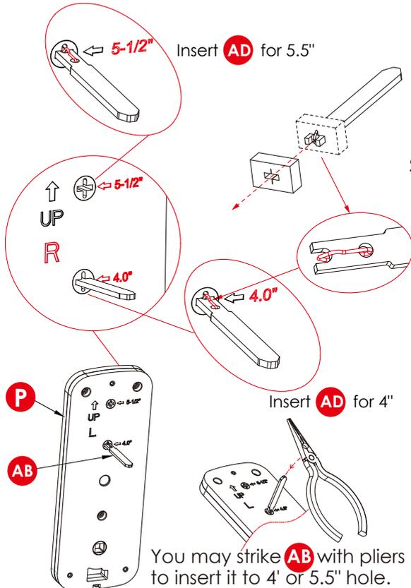
Select the correct side of the interconnection gear.
